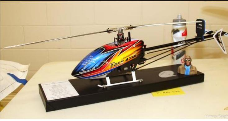
An electric heli entered in the ARF category by Frank Pilih. This is a new Align kit—a T-REX 470 featuring a new 470MX motor and including carbon fibre side frame plates.
