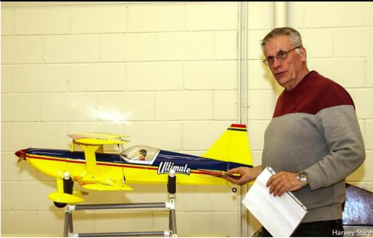
Terry Sears' Ultimate biplane was originally a glow powered kit, but Terry converted it to electric power. Terry also gave us a short run-down on the technical aspects of the model, as well as its expected flight characteristics. A fantastic looking model!
