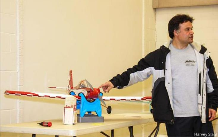
Aldo Agostini and his modified Sig Four-Star 40, which he converted to electric power. Other mods include a slightly more rounded tail and a new, stronger landing gear. Aldo made a mold of the nose area and mad various plastic cowls for the model.
