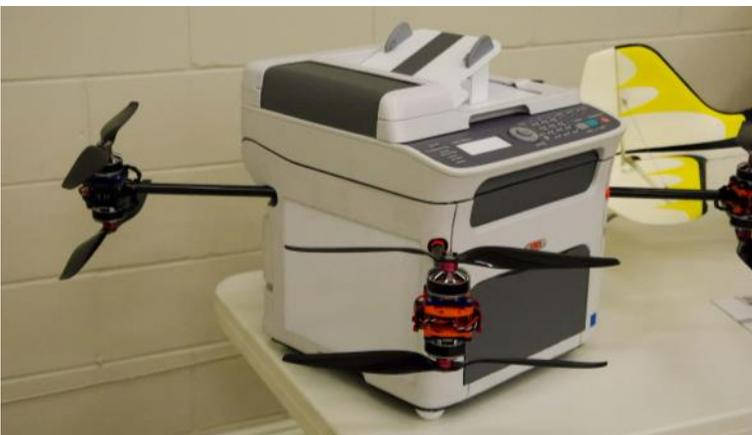
The 'flying printer' was the result of having a printer casing lying around, and the curiosity to see if it could be converted to a flying machine. The machine has eight independently controlled motors, as well having a flight controller that is capable of fully autonomous flight
