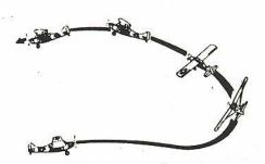
\* Falling Leaf: This manoeuver is essentially a continuously alternating series of left and right side slips, executed almost at the stall. To illustrate it, imagine a head-on view of the aircraft hanging from a string and swinging through an arc of about 60 degrees, like a pendulum. The speed towards you would be the absolute minimum necessary to prevent a complete stall, and the aircraft would be descending steadily in a series of sideways sweeps.
